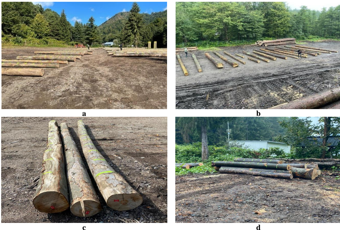
Fig. 1. Examples of wood arrangement during the field tests: a – Storage area 1 (S1, broadleaved), individual arrangement of logs in two groups (G1 and G2), and phone scanning activities; b - Storage area 2 (S2, resinous), individual arrangement of logs in one group (G3) and phone scanning activities; c – Storage area 1 (S1), bunched arrangement of logs in group 2 (G2), d – Storage area 1 (S1), an example of piled arrangement of the logs.
