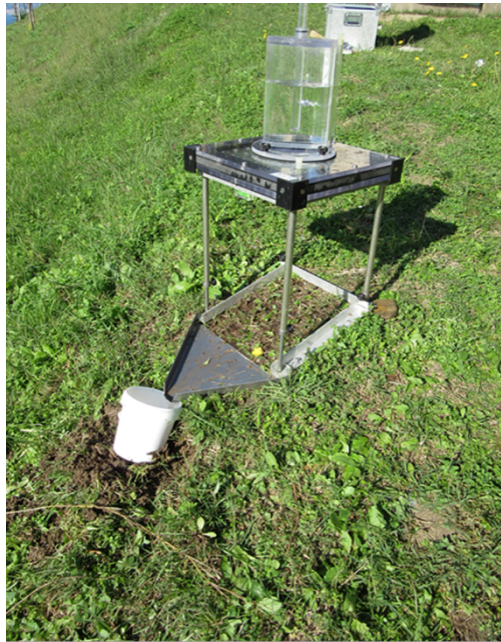
Figure 14 - A rainfall simulator (Eijkelkamp, Nederland).
