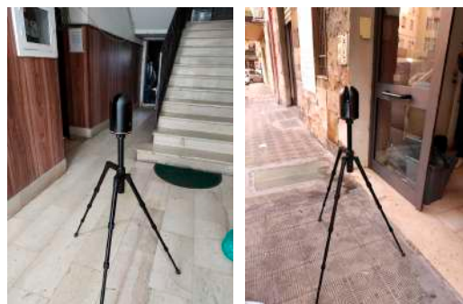
Figure 3. The survey phase with a laser scanner.
