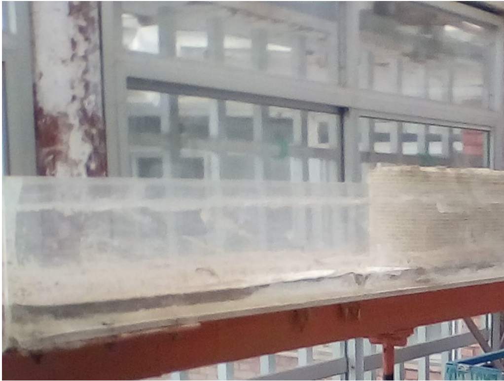
Figure 1 - Experimental flume used to simulate rill detachment on soil samples collected in Saravan Forestland Park (Guilan Province, Iran).
