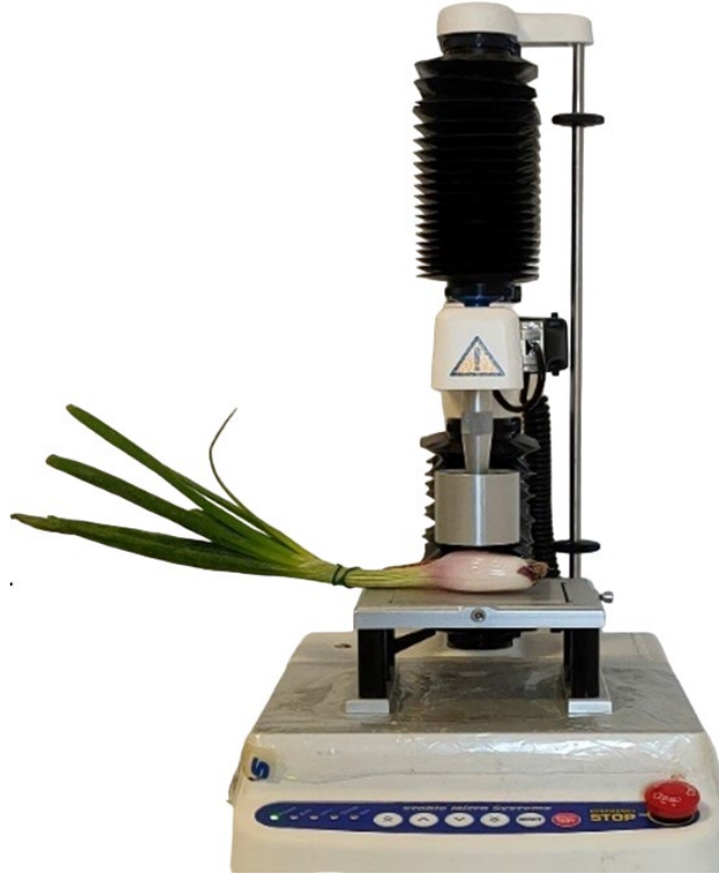
Fig. 2. Texture Analyser used during compression test.
