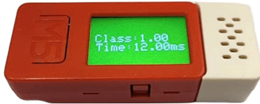
Figure 9. Classification results using M5C+. The screen shows the predicted class and the inference time in milliseconds.
