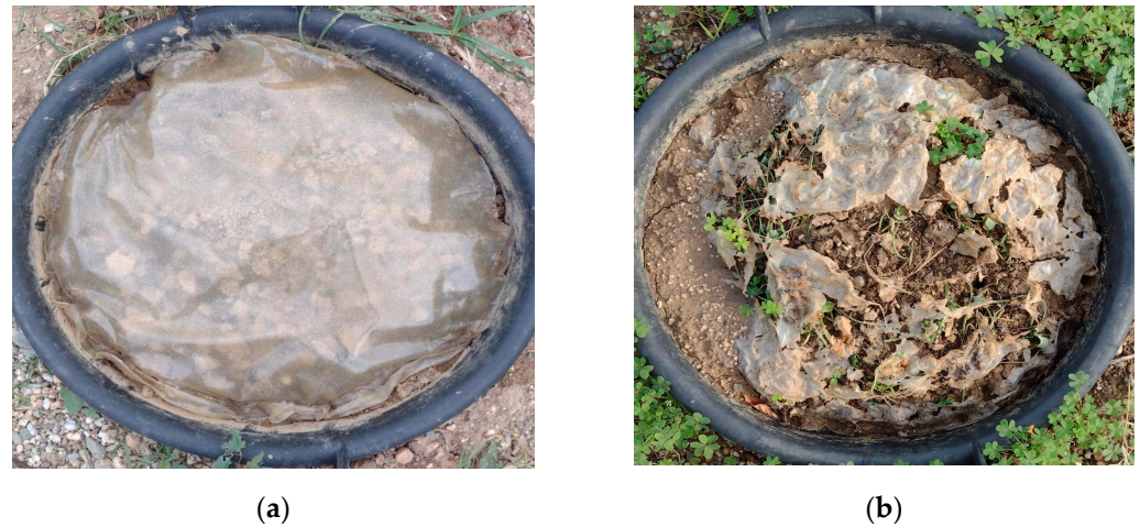
Figure 2. The BPMF mechanical collapse process: at the beginning of the pre-trial (a) and after 3-week exposure to field conditions (b).
