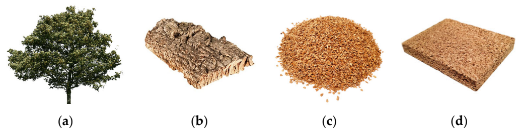
Figure 3. Corkboard production process: (a) cork tree: located in the municipality of Lamezia Terme (Italy), Calabria region; (b) debarked cork plank; (c) granulated cork; and (d) ecological cork panel. Source: Authors.
