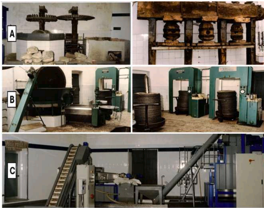
Fig. 3. Different Olive oil production installations that were successively implemented in the Olive Mill (OM): A) First generation, B) Second generation, C) Third generation.
