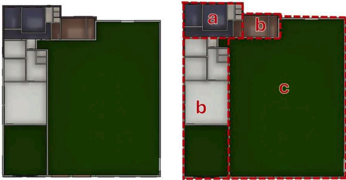
Fig. 5. The different sections position within the Olive Mill (OM): a) Adaptive reused administration section, b) newly constructed administration section, c) Operational area.
