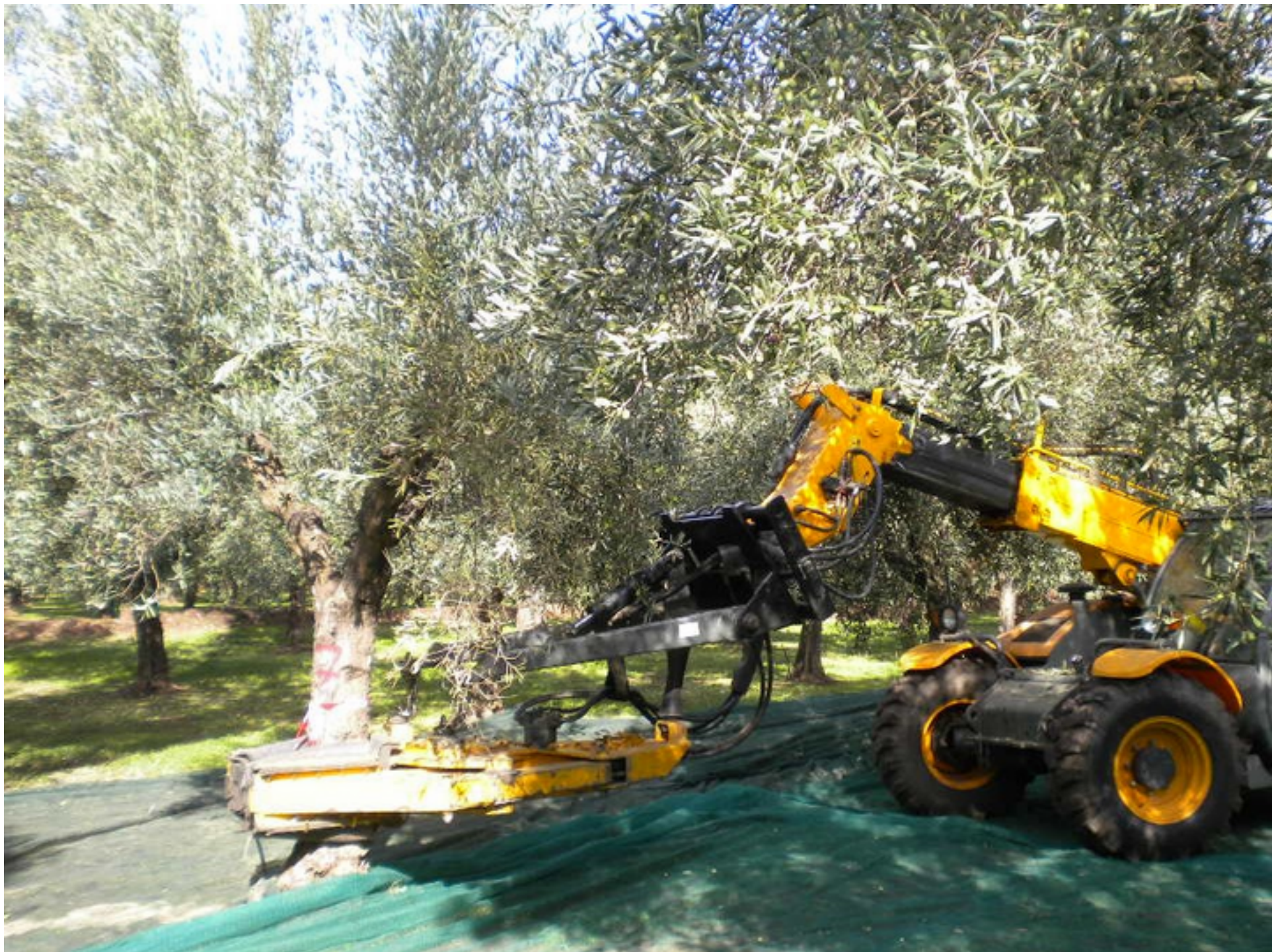
Figure 1: A self-propelled trunk shaker used in the harvesting of olives. Click here to download high resolution image
