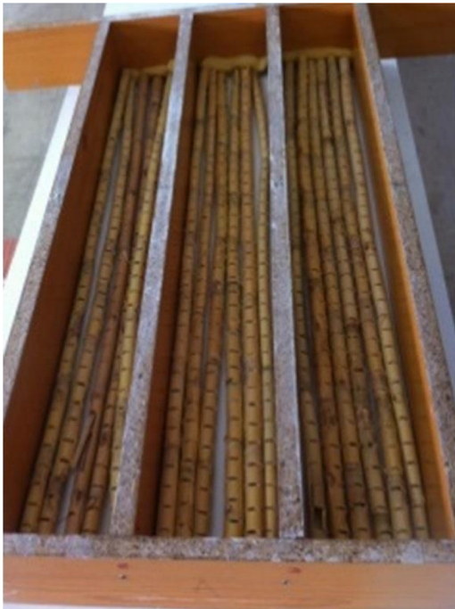
Fig. 5. Slotted reed inside the specimen mold.
