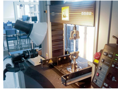
Figure 2. Experimental equipment used for the viscoelastic characterisation of the UHMWPE material
