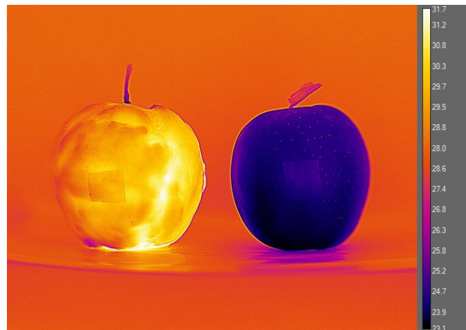
Fig. 4. Emissivity evaluation by black vinyl electrical tape.
