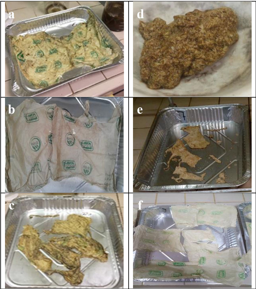
286 Figure 2. Digested compostable bags visual inspection; a) raw - mesophilic conditions – 15 days, b) 287 raw - mesophilic conditions – 30 days, c) raw - thermophilic conditions – 15 days, d) raw - 288 thermophilic conditions – 30 days; e) NaOH pre-treated - mesophilic conditions – 15 days, f) pre- 289 digested - mesophilic conditions – 15 days.
