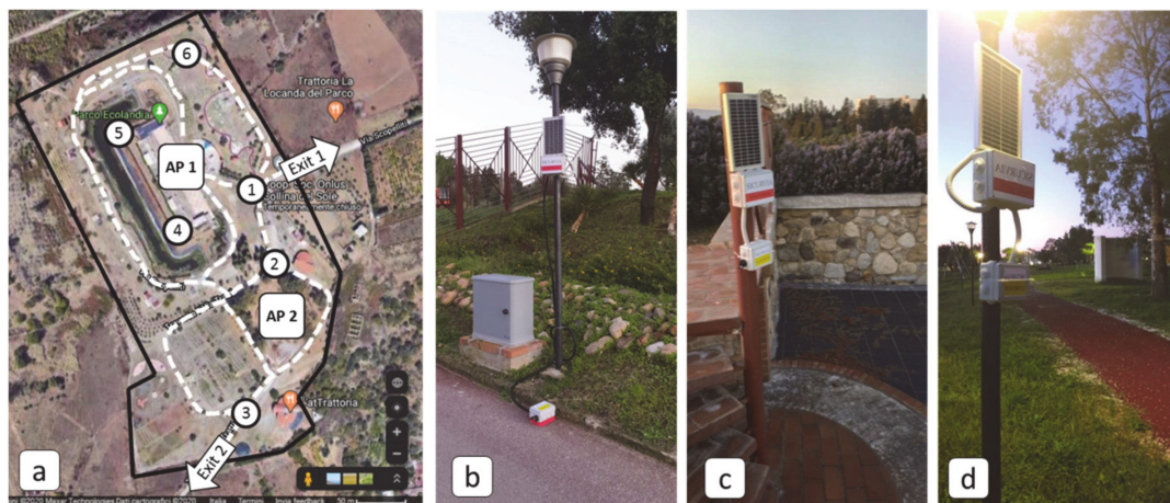
Figure 2. (a) Map of the theme park where the WSN was installed and three self-powered wireless sensing nodes installed on (b) a road pavement, (c) a masonry structure, and (d) a light pole in the park.
