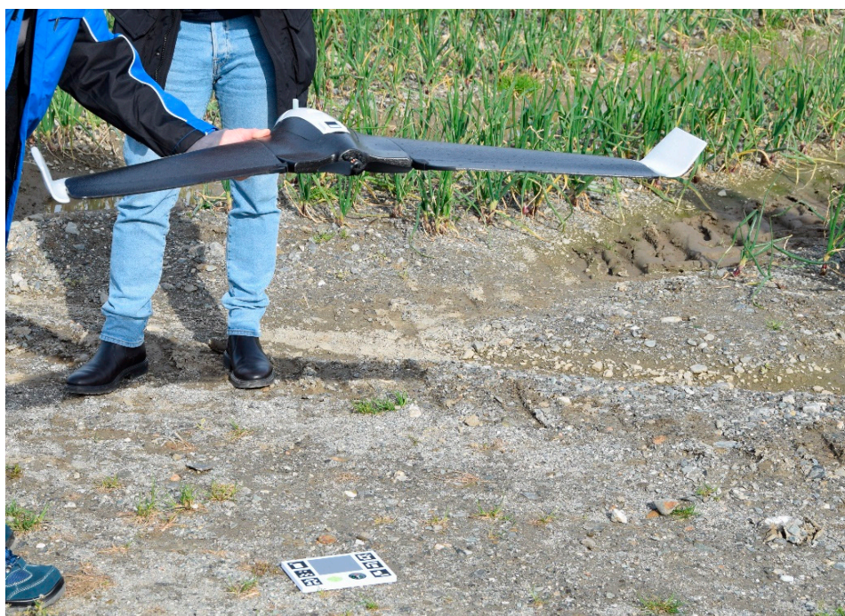
Figure 3. The Parrot Disco-Pro AG fixed-wing unmanned aerial vehicle (UAV) during the pre-flight calibration using the Parrot Sequoia calibration target.
