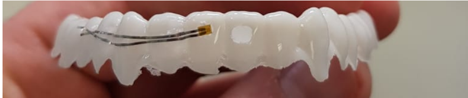
Fig. 5. Application of a strain gauge sensor in an intraoral appliance.
