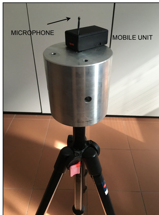
Figure 7. The MU used for the point grid measurement with its stand at z = 1 .
