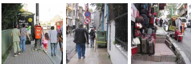
Bollards at minor street intersections and driveways indicate the high priority given to the vehicular traffic - that pedestrians have to yield. Unfortunately high kerbs generate a disrupted walking rhythm and unfortunate difficulties.
