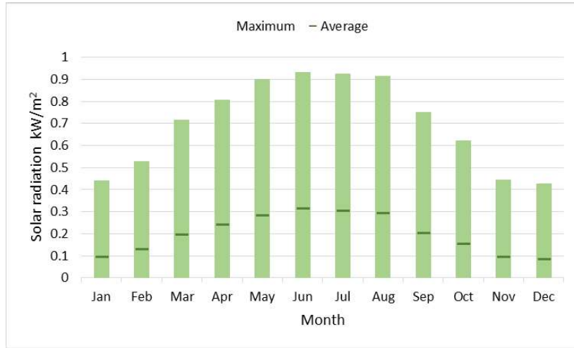
Figure 5 – Monthly maximum and average values of daily solar radiation on the horizontal
