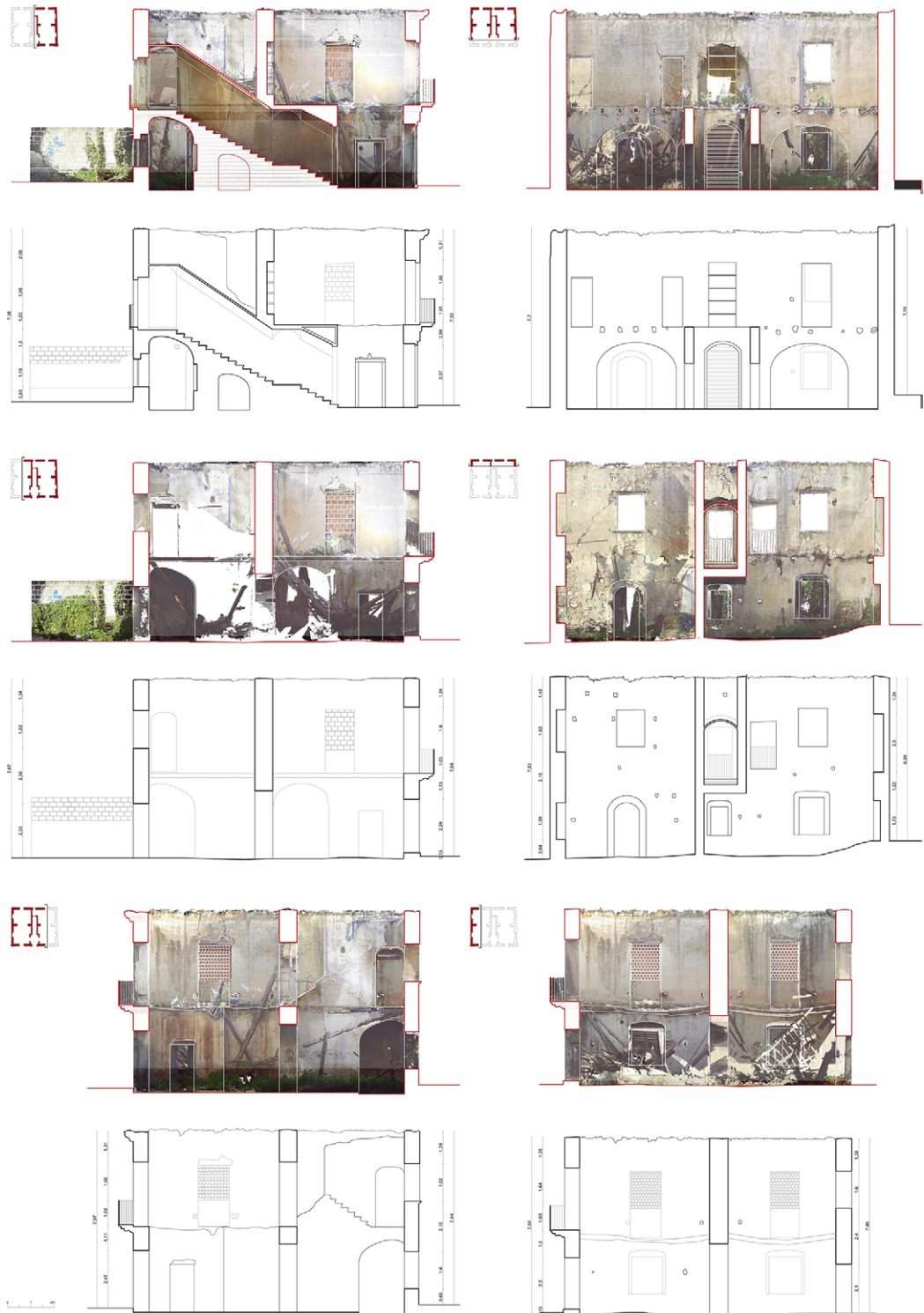
Fig. 8. Portanova Palace, Reggio Calabria. Drawing of sections from laser scanning. Drawings made under the guide of the author by Stefania Caporale, Francesca Maria Derenzo, Francesca Muscherà and Natali Sardone.
