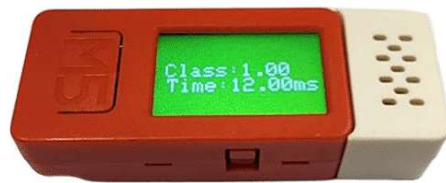
Fig. 4.15: OTA classification results displayed on the M5C+ device, including the predicted class and inference time.
