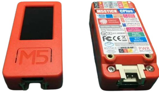
Fig. 4.6: M5Stick C Plus (M5C+) device used for environmental data acquisition and on-device OTA classification.
