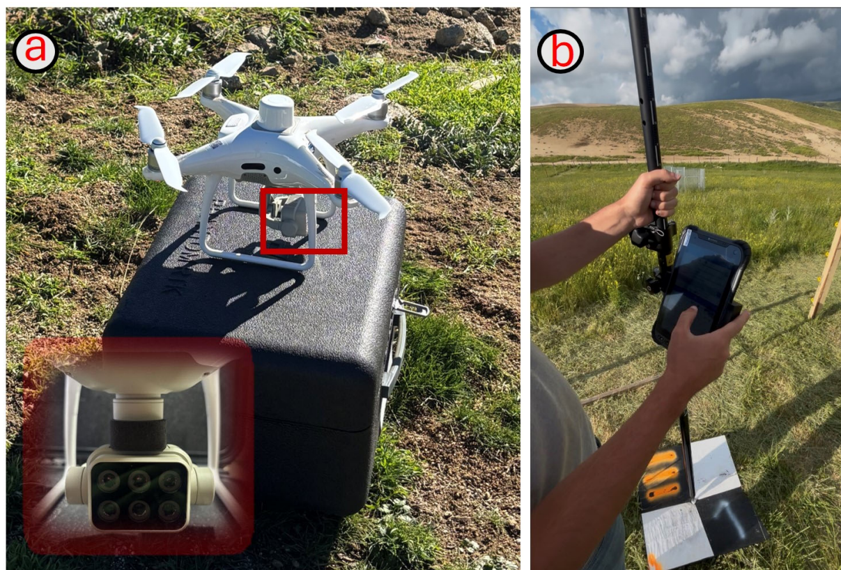
Figure 3. (a), DJI Phantom 4 Multispectral employed for aerial surveys. (b) Determination of the position of a ground control point (GCP).
