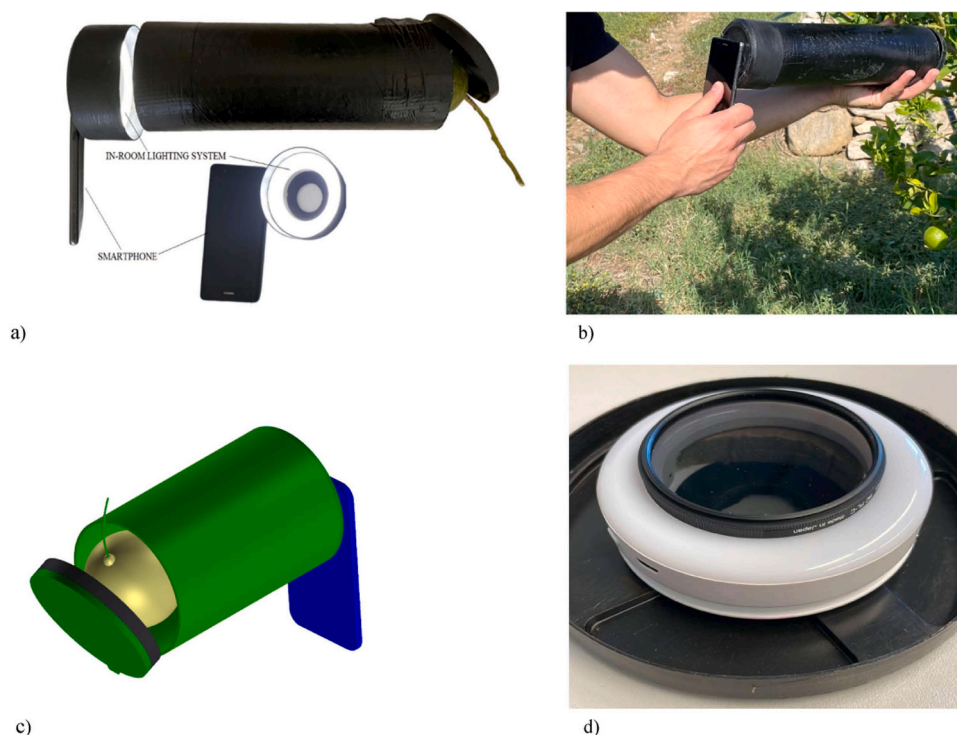
Fig. 1. Portable inspection chamber. a) Overall view; b) Field use; c) Graphical representation d) In-room lighting system.
