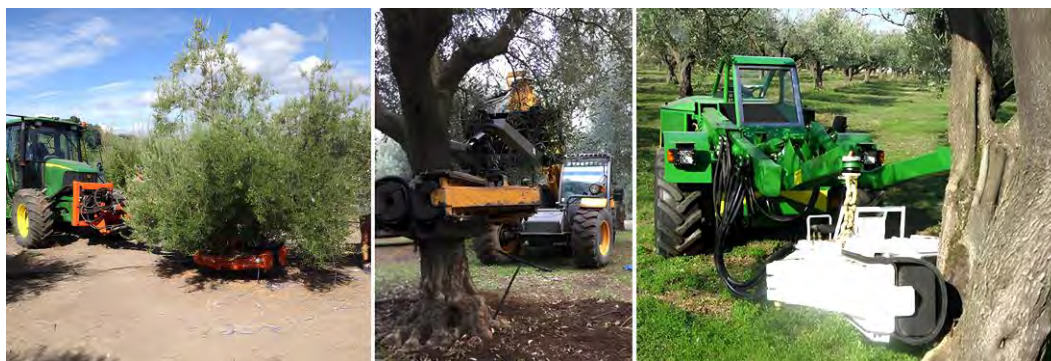
Figure 8. Self-propelled shaker in action on olive trees of different ages and dimensions: young ( on the left ), medium-aged ( in the centre ), and old ( on the right ). Note the differences in the capacity of the gripper to wrap around the trunk.
