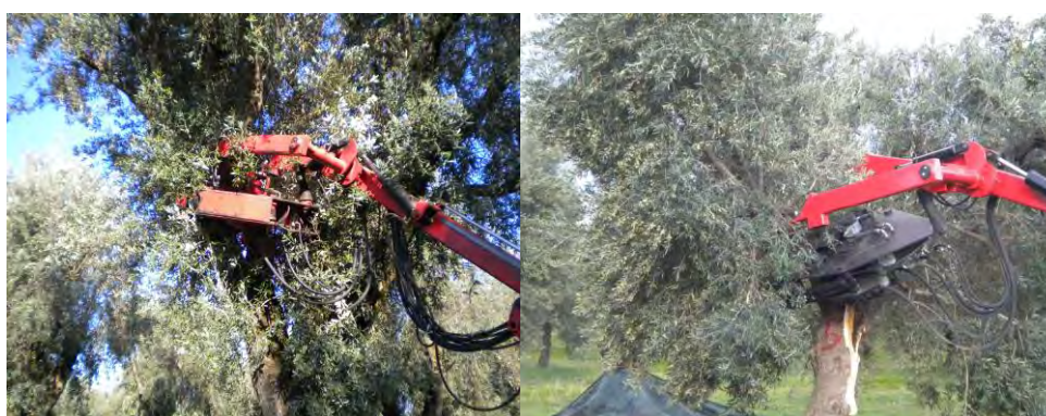
Figure 15. Example of issues in attaching the trunk shaker to the branches of ancient olive trees.
