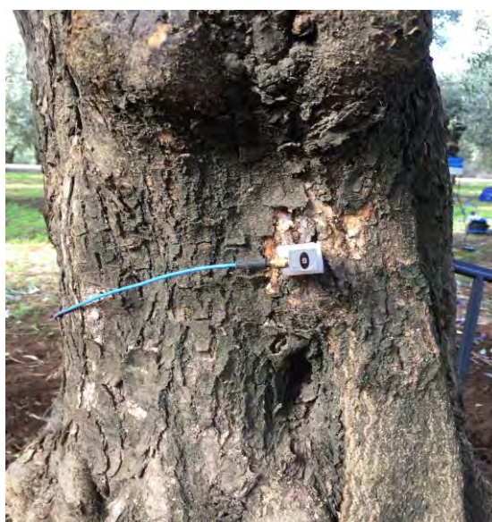
Figure 9. An accelerometer placed on the olive tree's trunk.
