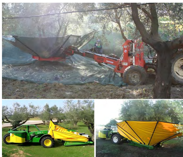
Figure 7. The top trunk shaker is equipped with a reversed umbrella mounted on a tractor. Below is a self-propelled trunk shaker with a closed and open reversed umbrella (on the (left) and the (right) , respectively).
