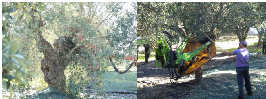
Figure 12. Difficulty in using oversized heads during work.
