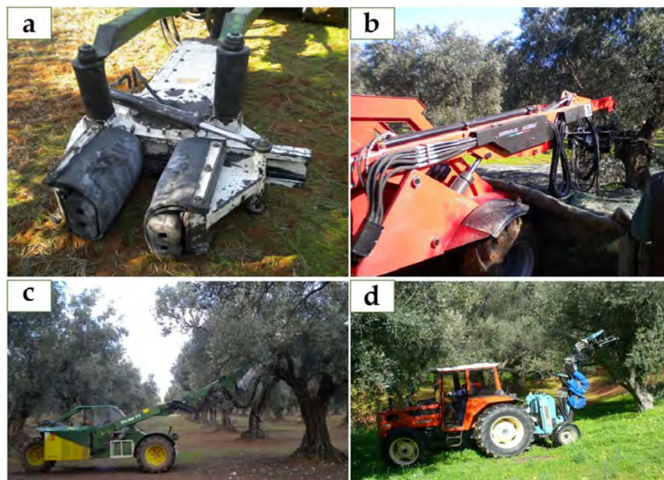
Figure 1. (a) Trunk shaker's gripping organ (clamp); (b) pivoting arm of variable length; (c) self-propelled trunk shaker; (d) trunk shaker coupled to a tractor.
