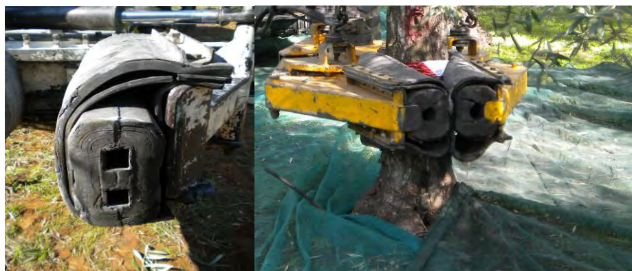
Figure 11. Attachment materials and their wear level.
