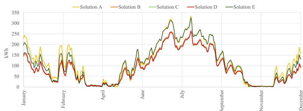
Figure 8. Energy consumption by the HVAC for different wall living solutions.
