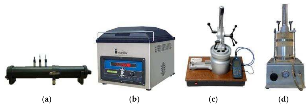
Figure 5. Instruments used to derive (a) the sound absorption coefficient, (b) the porosity, (c) the airflow resistivity, and (d) the hydraulic permeability of the samples used in this study.
