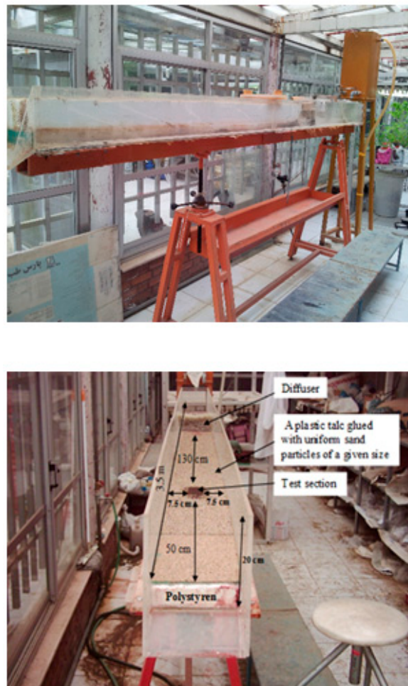
Figure 2. The experimental flume used to measure the rill detachment capacity under four land uses in the Saravan watershed (Northern Iran) [45,46].
