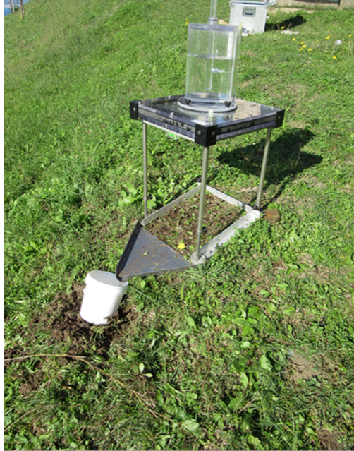
Figure 14 - A rainfall simulator (Eijkelkamp, Nederland).
