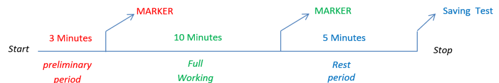
Figure 1. Sampling test scheme adopted to monitor the energy consumed. Three periods can be distinguished: preliminary period of 3 min (in red on the left); the main period of full working of 10 min (in the centre in green); the rest period of non-work with a duration of 5 min (in blue on the right).
