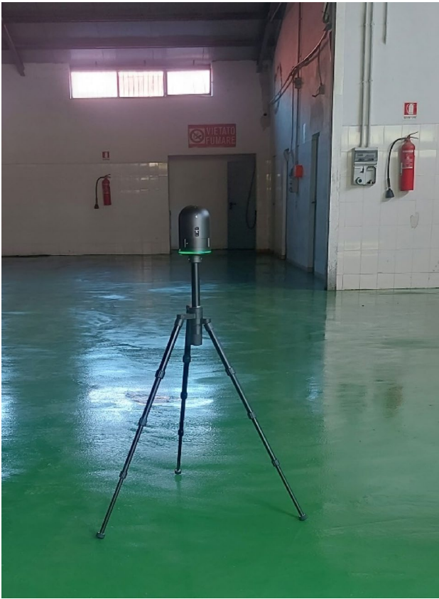
Fig. 3 Leica BLK360 terrestrial laser scanner (TLS) used for the survey
