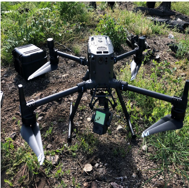
Fig. 4 Uncrewed Aerial Vehicle (UAV) DJI Matrice 300 RTK used for the survey
