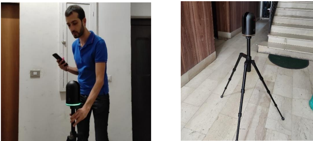
Figure 2. The survey phase with laser scanner.
