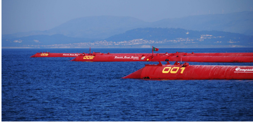
Fig. 1.5: Pelamis WECs installed off the coast in the North of Portugal. From Ref. [4]
