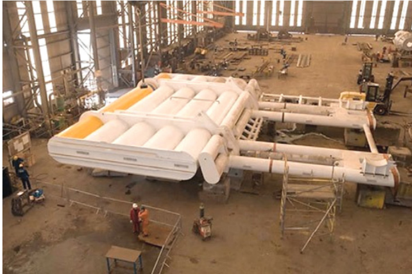
Fig. 1.6: Oyster prototype. From Ref. [4]
