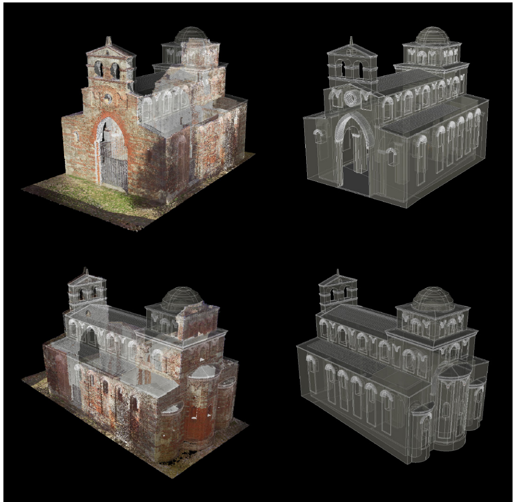
Fig. 10. Santa Maria de' Tridetti, Staiti, 11th-12th century. Overlay of laser scan point cloud and 3D model with hypothesis of original configuration. Laser scanner survey by Marinella Arena, Daniele Colistra and Domenico Mediati. 3D model and graphic processing by the author.
