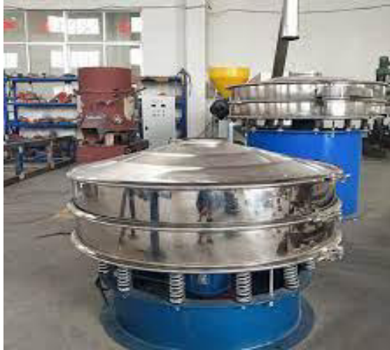
Figure 2.14 Example of multi-sieve vibrator with gradually finer sieve sizes
