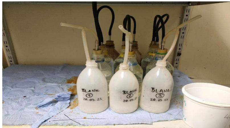
Figure 6.2 Reactors placed inside the climatic chamber at 37 °C
