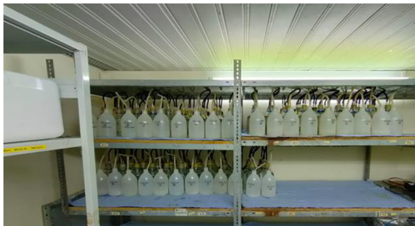
Figure 3.12 Climate cell set at a temperature of 37 °C to favour the mesophilic environment.
