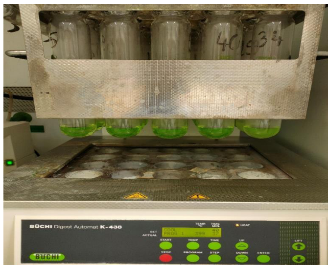
Figure 3.3 Samples subjected to thermal cycling for TKN analysis.
