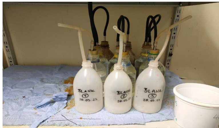
Figure 5.2 Reactors placed inside the climatic chamber at 37 °C
