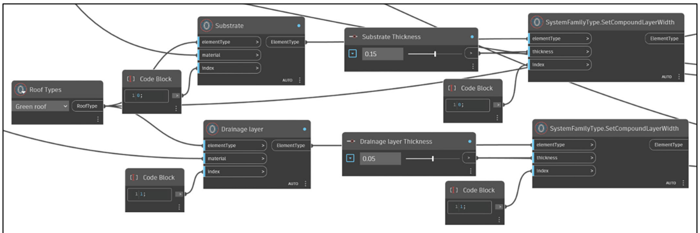
Figure 5. Layer creation into the green roof type and parametric thickness modelling.
