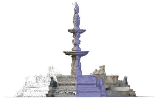
Figure 9: Survey data processing phases. From point cloud to textured mesh.
