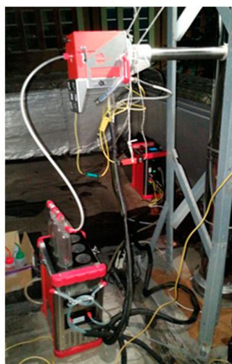
Figure 3. Sugar sampling system: DADOLAB HP5 probe containing the fiber glass filter for the solid component and the thermostated impingers for the sampling of the volatile fraction.
