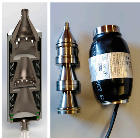
Figure 4. Multistage inertial impactor for PM fraction sampling.
