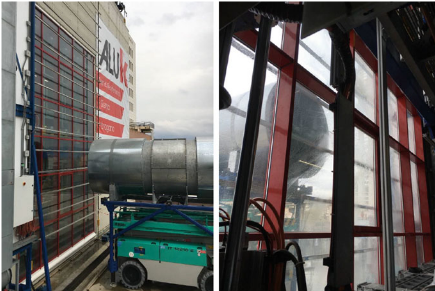
Fig. 62.1 Example of hurricane simulation on a curtain wall. Credit TCLab
