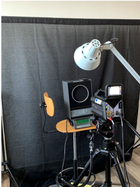
Fig. 3. Thermal camera and blackbody. This figure shows the instrumentation used for experimentation.
