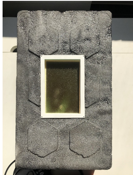
Figure 3. Test box for rapid measurement of optical characteristics of the greenhouse covering. It is portable and enables measurement of the parameters of the greenhouse covering under real conditions.
