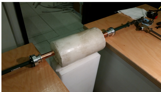
Fig. 5.45. Setup with paraffin wax cylinder between horns
