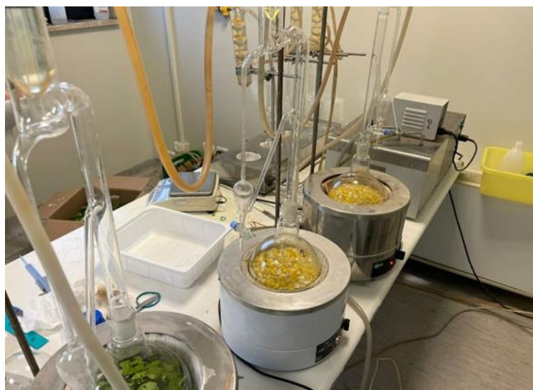
Figure 2.6 Hydro-steam-distillation of bergamot fruits.
