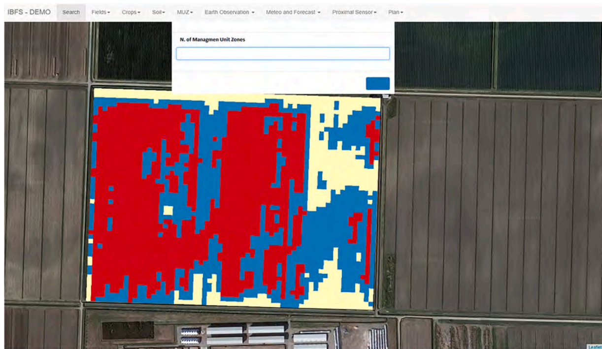
Fig. 8. An example of mapping 3 Management unit zones (MUZs), delineated for one field by the Fuzzy c-means algorithm on Maximum Value Composite (MVC) data superimposed on a satellite base map.
