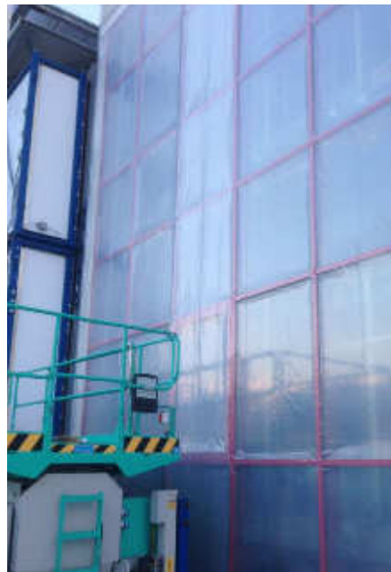
Fig. 27 - Simulazione carico e pressione del vento / Load and pressure wind simulation (Source: Authors' elaboration).
