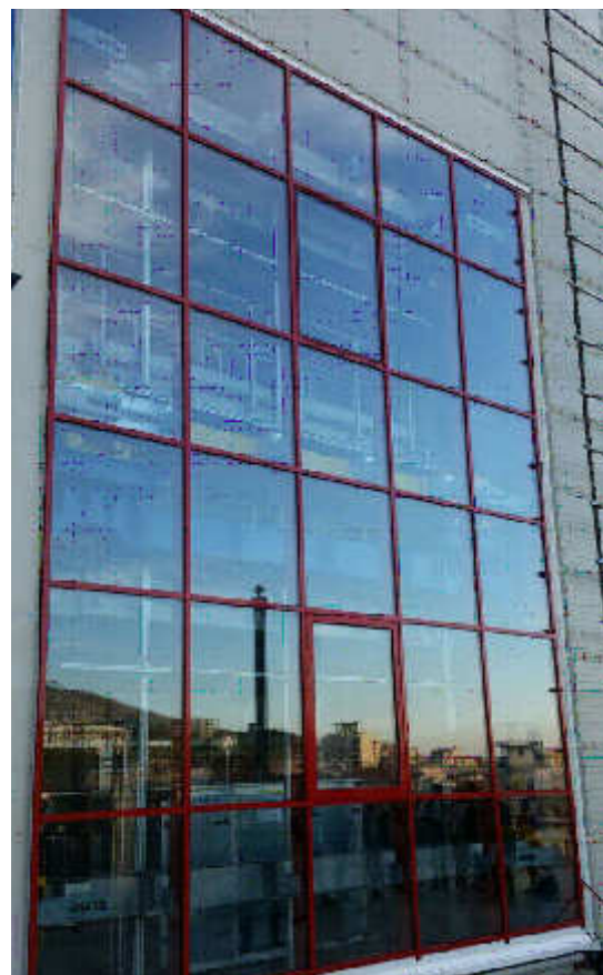
Fig. 24 - Campione sottoposto a prova nell'assetto sperimentale: Full Scale Mock-Up / Sample tested in the experimental setup: Full Scale Mock-Up (Source: Authors' elaboration).
