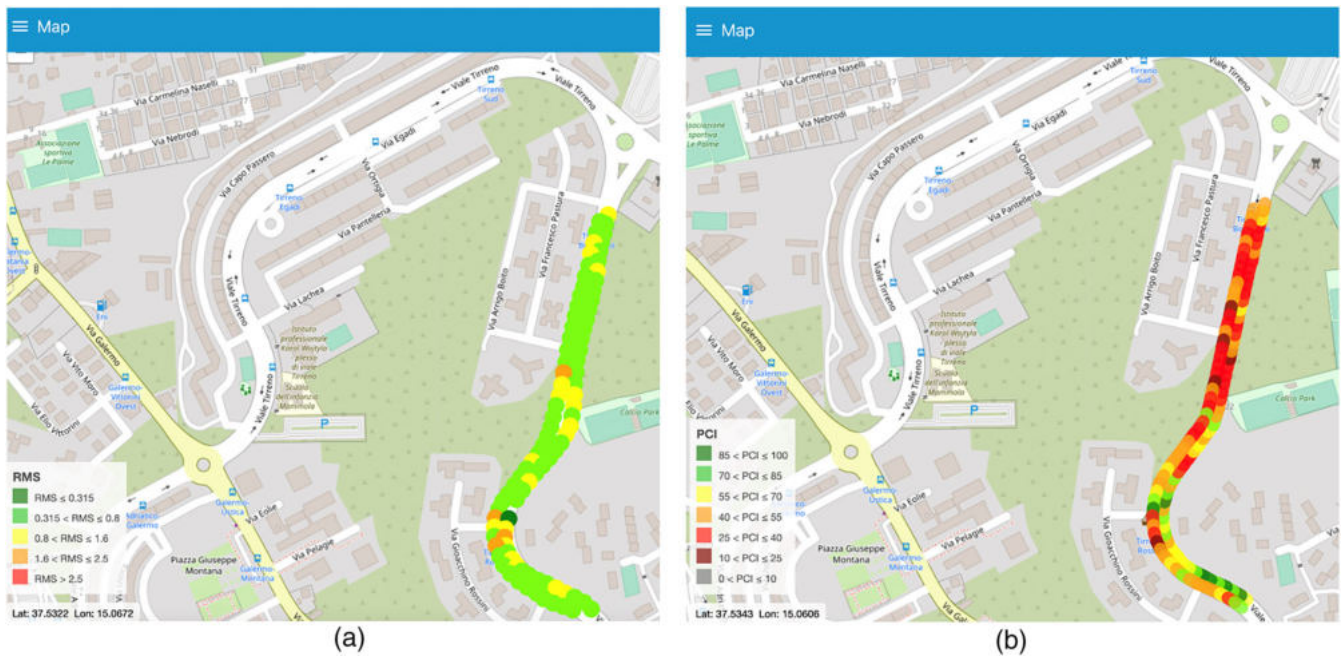
FIGURE 11 Condition data shown in the web-platform: (a) RMSw; (b) PCI
