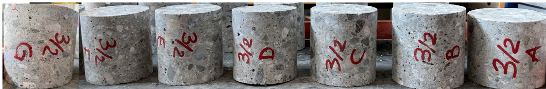
Figure 4. Cores extracted from concrete wall via drilling: (a) Specimens 1/1 (a–g); (b) Specimens 1/2 (a–g); (c) Specimens 1/3 (a–g); (d) Specimens 2/1 (a–g); (e) Specimens 2/2 (a–g); (f) Specimens 2/3 (a–g); (g) Specimens 3/1 (a,b,d–g); (h) Specimens 3/2 (a–g). All cores have diameters of 94 mm and variable heights (from 85 to 103 mm).
