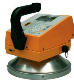
Figure 6: NCAT Asphalt Field Permeameter
