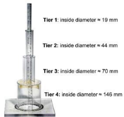
Figure 6: NCAT Asphalt Field Permeameter
