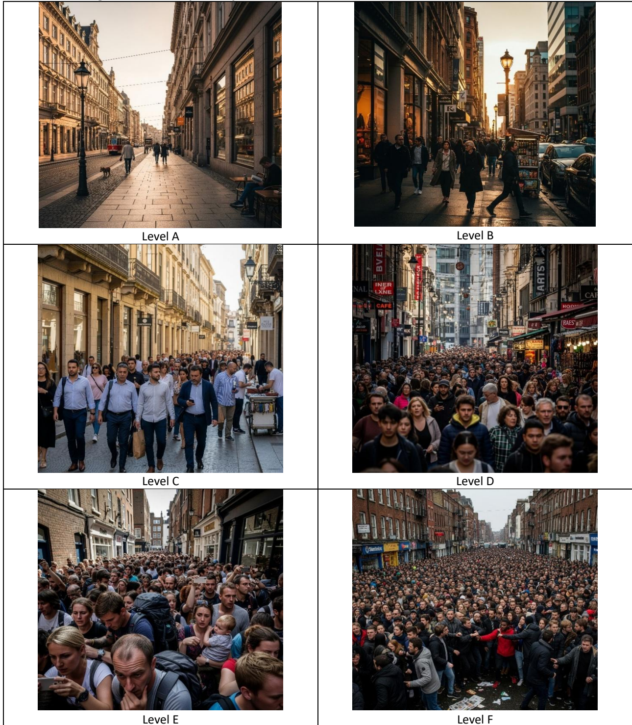
Figure 2.2 - Examples of pedestrian infrastructures in different LoS conditions.
