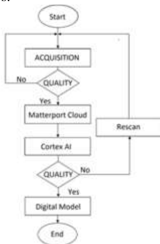
Fig. 4: illustrates the process of creating the digital model
